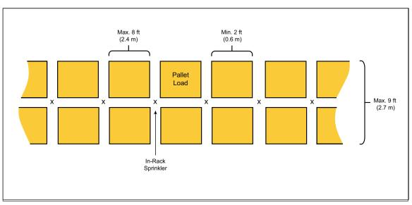
Fig. 12. Plan view of IRAS(E) horizontal in-rack sprinkler arrangement for double-row racks having a maximum depth of 9 ft (2.7 m)
