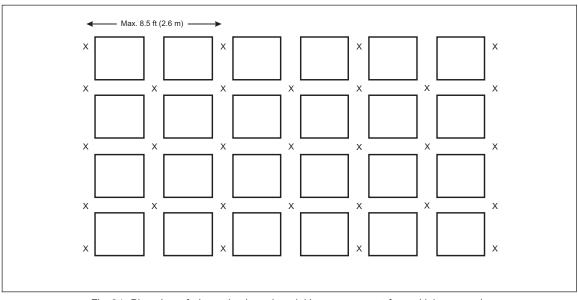
Fig. 21. Plan view of alternative in-rack sprinkler arrangement for multiple-row racks
