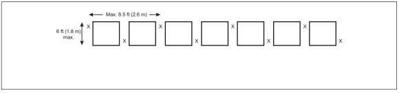
Fig. 19b. Plan view of alternative in-rack sprinkler arrangement for single-row racks up to 6 ft (1.8 m) deep
