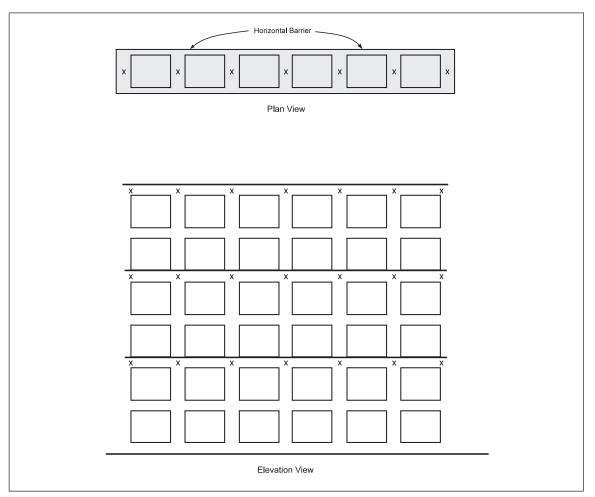
Fig. 16. Fire Protection Scheme 8-9A within single-row racks
