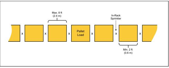
Fig. 11. Plan view of IRAS(E) horizontal in-rack sprinkler arrangement for single-row racks
