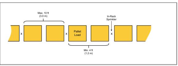
Fig. 8. Plan view of IRAS(EO) horizontal in-rack sprinkler arrangement for single-row racks
