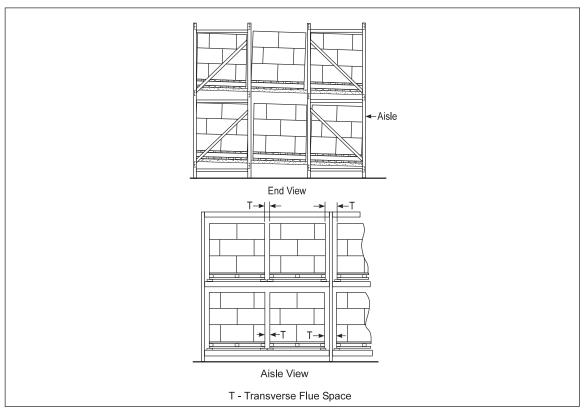
Fig. A-8. Flow-through pallet rack
