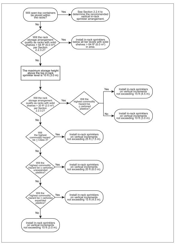
Fig. 15. Recommended vertical in-rack sprinkler increments
