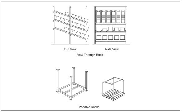
Fig. A-10. Flow-through and portable racks
