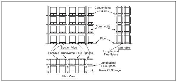
Fig. A-1. Typical double-row (back-to-back) rack arrangement
