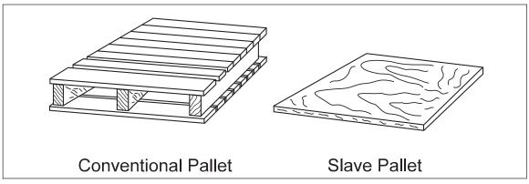
Fig. A-2. Typical wooden pallets
