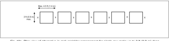
Fig. 19a. Plan view of alternative in-rack sprinkler arrangement for single-row racks up to 3 ft (0.9 m) deep
