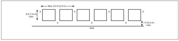
Fig. 19c. Plan view of alternative in-rack sprinkler arrangement for single-row racks up to 6 ft (1.8 m) deep located against wall
