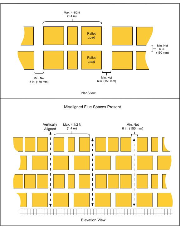
Fig. 2g. Acceptable flue space arrangement for double-row racks, Option 4
