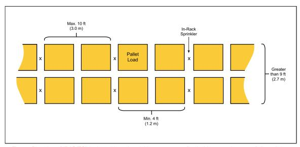
Fig. 9. Plan view of IRAS(EO) horizontal in-rack sprinkler arrangement for double-row racks up to 9 ft (2.7 m) deep
