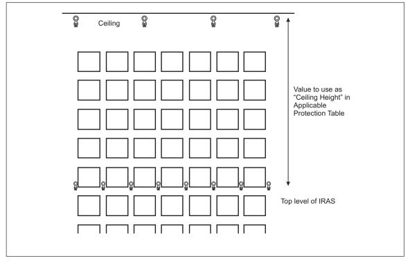
Fig. 22. Determining ceiling height in applicable protection table
