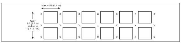
Fig. 20b. Plan view of alternative in-rack sprinkler arrangement for double-row racks up to 12 ft (3.7 m) deep
