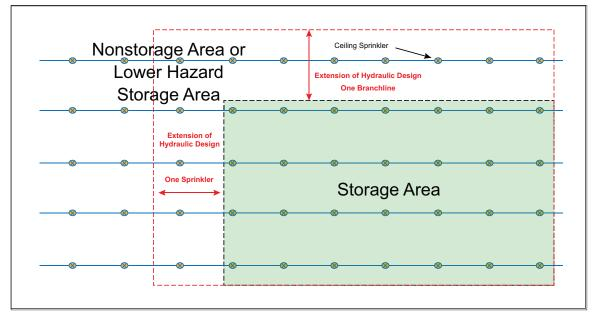
Fig. 21. Extension of hydraulic design
