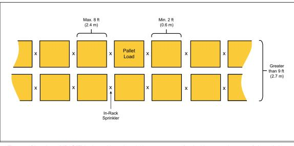
Fig. 12a. Plan view of IRAS(E) horizontal in-rack sprinkler arrangement for double-row racks over 9 ft (2.7 m) deep
