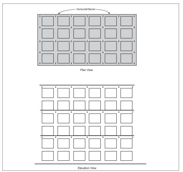
Fig. 18. Fire Protection Scheme 8-9A within multiple-row racks
