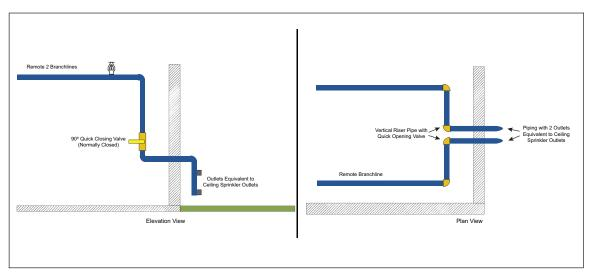
Fig. A-13. Example arrangement of an inspector's test connection for a dry sprinkler system design using 2 sprinklers on the most remote 2 branchlines (4 sprinklers total)
