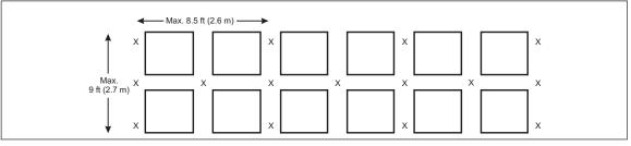
Fig. 20a. Plan view of alternative in-rack sprinkler arrangement for double-row racks up to 9 ft (2.7 m) deep
