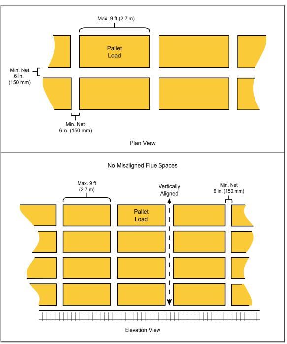
Fig. 2e. Acceptable flue space arrangement for double-row racks, Option 2
